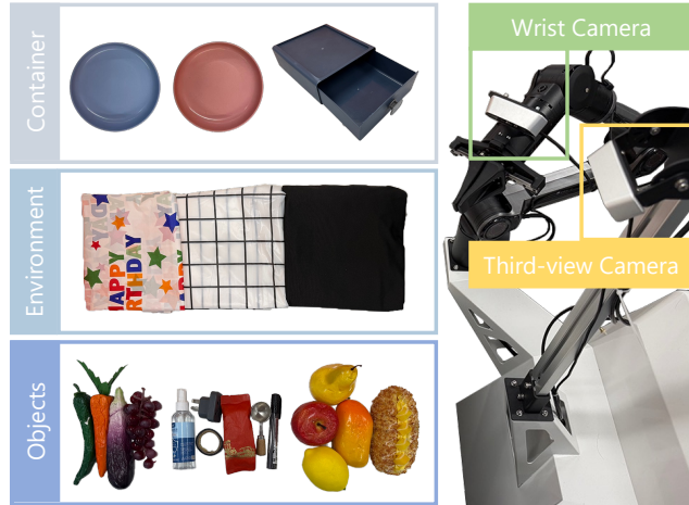
Figure 12: Real-world platform, containers, objects, and background variations used in our real-world evaluations.
